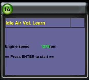
9.If Finished! shows on screen, it means Idle Air Volume Learning performs successfully.
